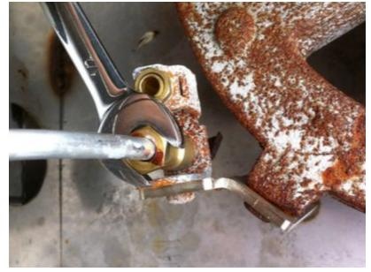
c. Carefully remove the aluminum tubing:
