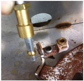
d. Use needle nose pliers to remove pilot orifice.
