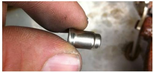
f. When clean and dried, a tiny hole will be seen through the orifice.
